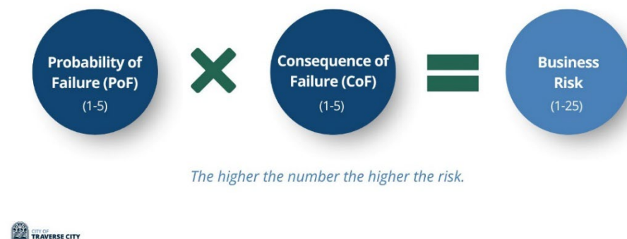
Figure 30: Risk of Failure Analysis Calculation
