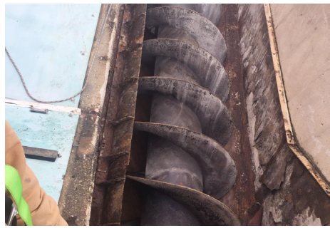
Before upgrade. Out of service because screw body was cracked.
