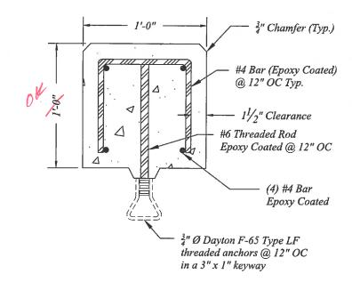
3/4" Ø F-65LF Threaded Insert For Tieplate Connection Typ. - (2 Places)
