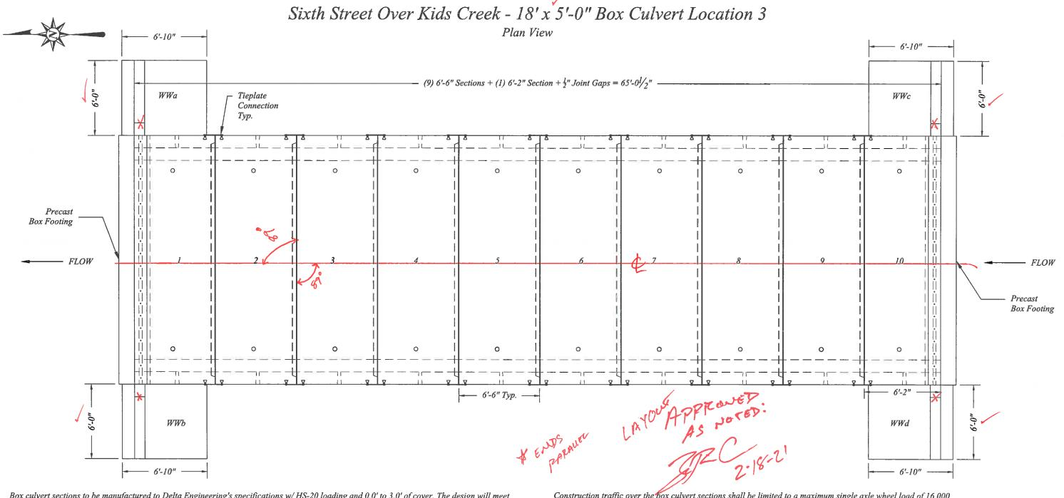
Box culvert sections to be manufactured to Delta Engineering's specifications w/ HS-20 loading and 0.0' to 3.0' of cover. The design will meet all other applicable ASTM C-1433 Specifications.
