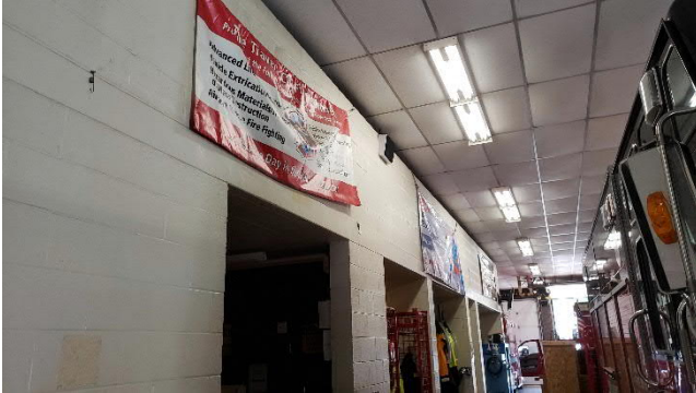
Figure M1.13 Apparatus Bay (no gas detection or exhaust system)
