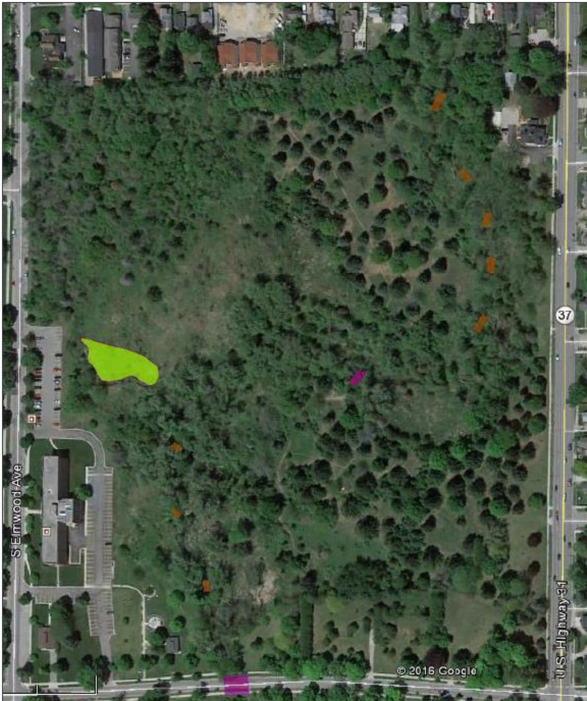
Figure 23. Recommended riffle improvements (in brown), culvert replacements (in purple) and floodplain storage improvements (in green) on Kids Creek from 11th Street to 7th Street
