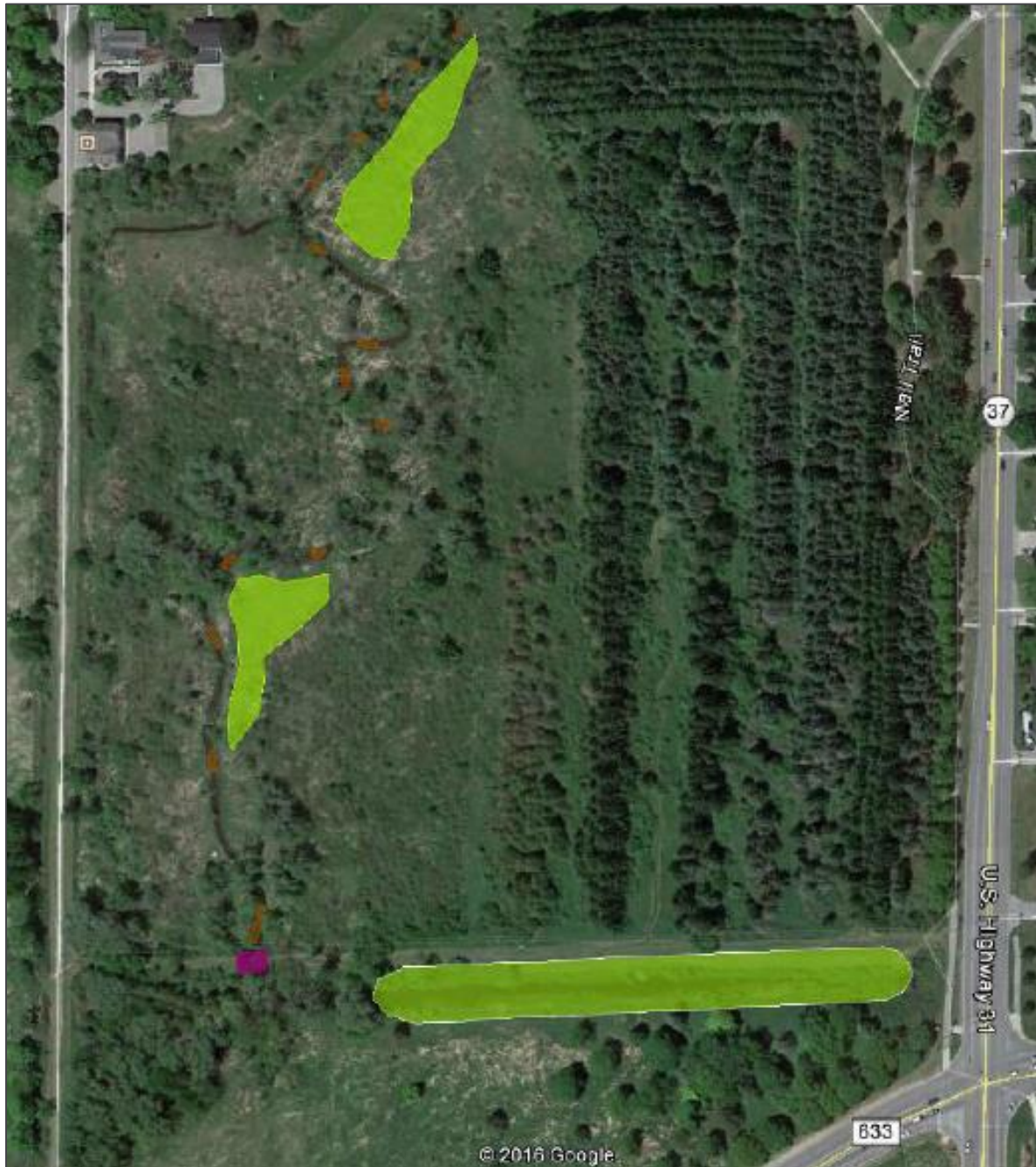
Figure 22. Recommended riffle improvements (in brown), culvert replacements (in purple) and floodplain storage improvements (in green) on Kids Creek from Silver Lake Street to above 11th Street
