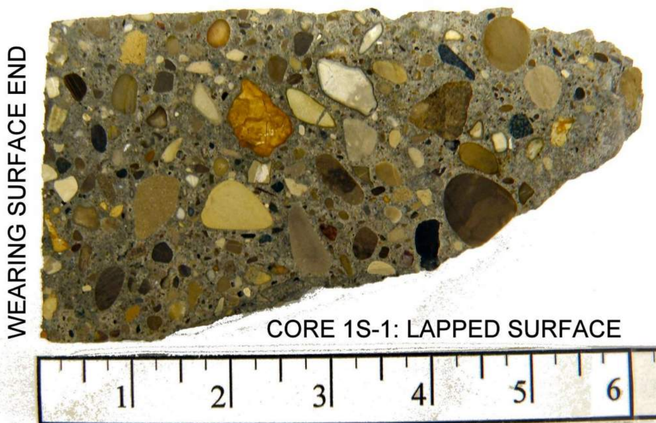
Figure 8. This view shows a lapped surface of one of the Core 1S-1 pieces from the compressive strength test. Features and properties of the core concrete are described below.
