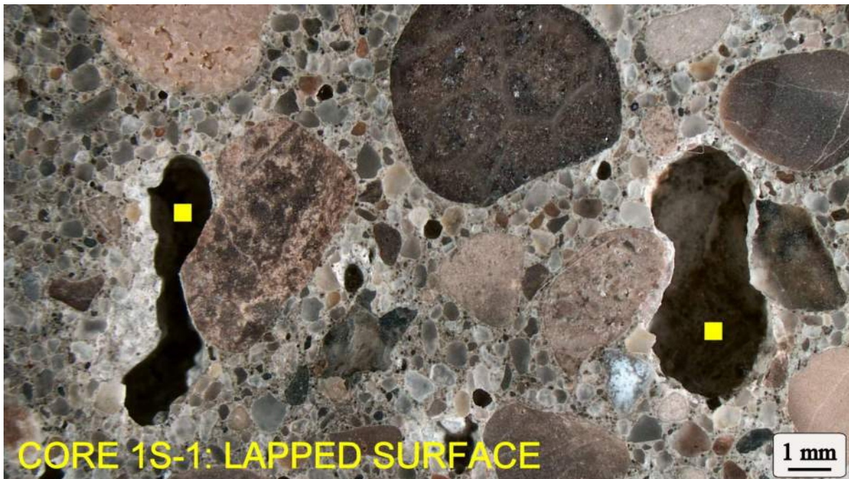
Figure 12. Photograph, taken at a magnification of 7X, on a lapped surface of Core 1S-1, showing two of the consolidation voids that are present in a minor amount in the core. Other than these innocuous artifacts, the core concrete is well-consolidated.
