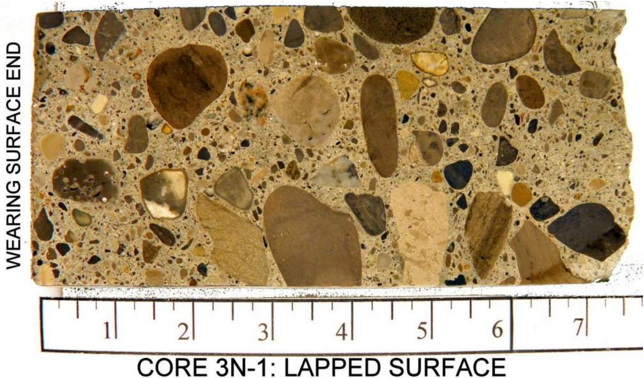
Figure 4. This lapped surface of Core 3N-1 shows the appearance of the concrete. Features and properties of the core concrete are described below.
