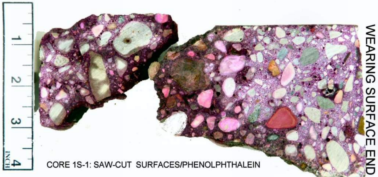
Figure 9. This view shows the appearance of saw-cut surfaces of two pieces of Core 1S-1, following the application of phenolphthalein solution. Features of interest are described below.
