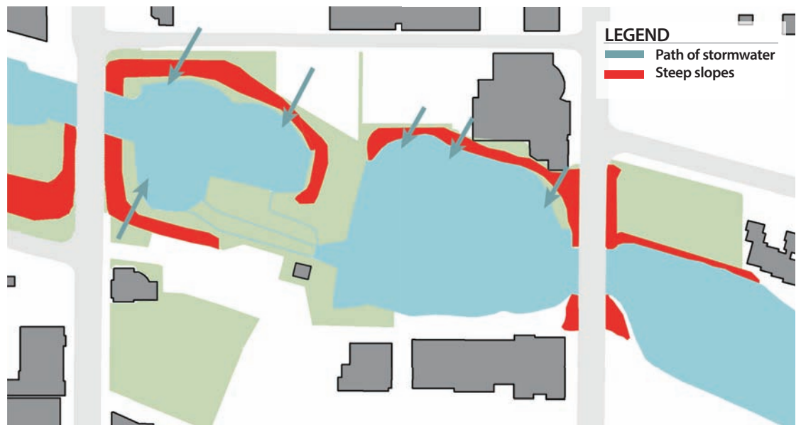
Figure 48: Ecological Conditions. Stormwater enters the park from the neighboring roads and parking lots, moving quickly down steep banks toward the river. Accessibility and ecological interventions should be considered at these points.
