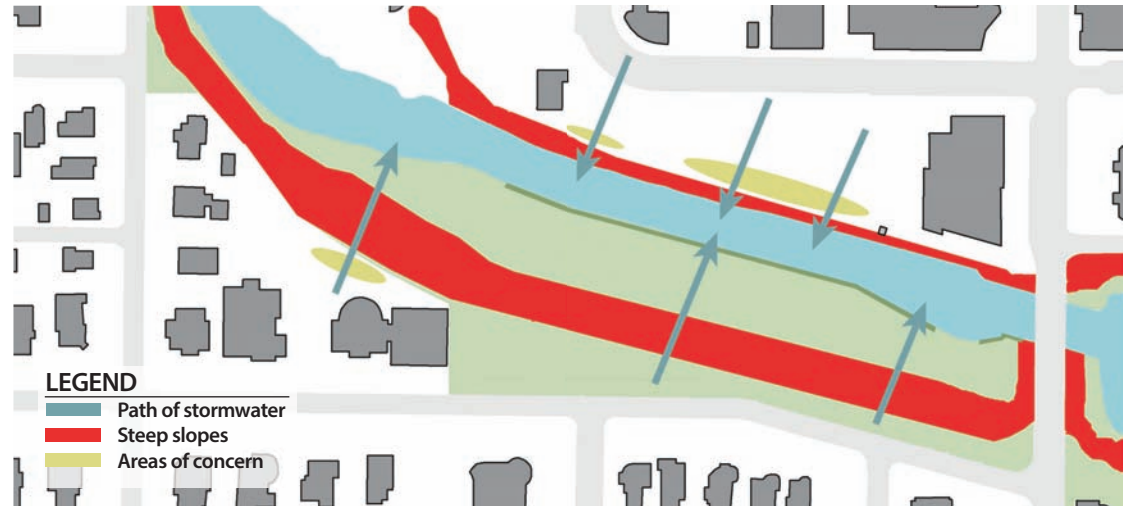
Figure 44: Ecological Conditions. Stormwater enters the park from the neighboring roads and parking lots, moving quickly down steep banks toward the river. Areas of concern are highlighted where rain gardens could prevent further erosion and treat stormwater.
