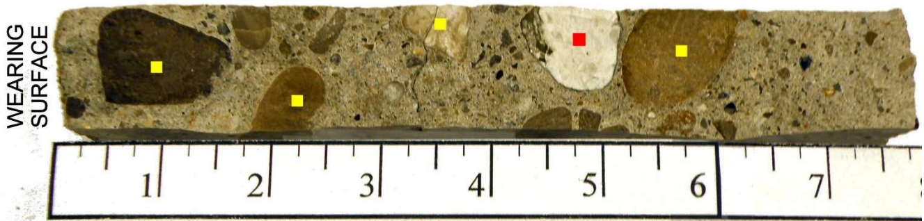
Figure 7. This view shows the appearance of the fracture surface that was intentionally created in Piece Z of Core 3N-1, in the ASTM C496 splitting tensile test. All of the coarse aggregate particles (dots on several) in the view fractured in the test, rather than pulling out intact. The red dot is on a chert aggregate particle that shows evidence of ASR activity (discussed in a later section). Other features of interest are discussed below.
